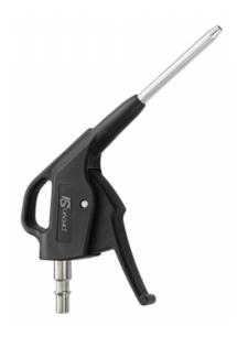
Blowing force (at 6 bar Dynamic pressure (at Air consumption (at 6 Sound level (at 6 bar (g)) 10 mm at 6 bar (bar)) bar (Nm3/h)) (dBA)) 390 2.2 20 89 Max operating Temperature Construction Highlight -15°C to +70°C Polyamide composite body Compact pressure 12 bar Connection Built-in adaptor
