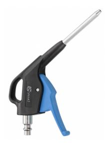
Blowing force (at 6 bar Dynamic pressure (at Air consumption (at 6 Sound level (at 6 bar 10 mm at 6 bar (bar)) bar (Nm3/h)) (dBA)) (g)) 390 2.2 20 89 Max operating **Temperature** Construction Highlight -15°C to +70°C Polyamide composite body Compact pressure 12 bar Connection Built-in adaptor
