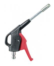
Air consumption (at 6 Blowing force (at 6 bar Dynamic pressure (at Sound level (at 6 bar (g)) 10 mm at 6 bar (bar)) bar (Nm3/h)) (dBA)) 248 2.3 13 85 Max operating **Temperature** Construction Highlight -15°C to +70°C Polyamide composite body Compact pressure 12 bar Connection Built-in adaptor
