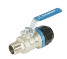
For pipe OD (mm) **BSPT** male thread **Technology** Operating pressure R 1/2 PPS Grip Concept 0 to 16 bar Vacuum capability **Temperature** Construction Highlight -20°C to +80°C Scalable system -0.98 bar (vacuum 98%) Pipe and fittings: alu. Meets standards PED REACH
