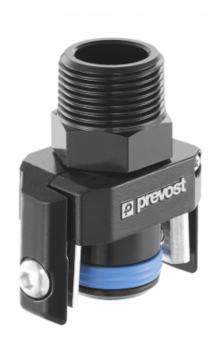
For pipe ID (mm) **BSPP** male thread Operating pressure **Technology** 25 G 3/4 PPS Grip Concept 0 to 16 bar Vacuum capability **Temperature** Construction Highlight -20°C to +80°C -0.98 bar (vacuum 98%) Pipe and fittings: alu. Scalable system Meets standards PED REACH
