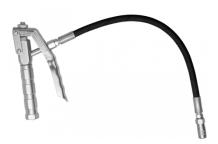
Technology Description Operating pressure Outlet pressure Distribution gun Piston dual action 3 to 7 bar 406 bar (air pressure at 7 bar) **BSPP** female thread BSPP male thread Flow rate Pressure ratio Air inlet: G 1/4 900 g/min (for air pressure 6 58:1 Grease outlet: G 1/4 bar)
