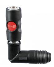
NPT female thread **Technology** Operating pressure Flow rate at 6 bar 3/8" FNPT "One push" safety system 2 to 12 bar 2028 I/min ( $\Delta P = 0.6$  bar) (avoids hose whip) **ID** Passage Construction Highlight **Temperature** 8 mm -15°C to +70°C Anti-static Non scratch Composite body
